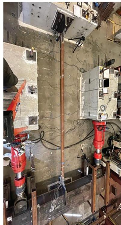
(b) Setup with a specimen in place
