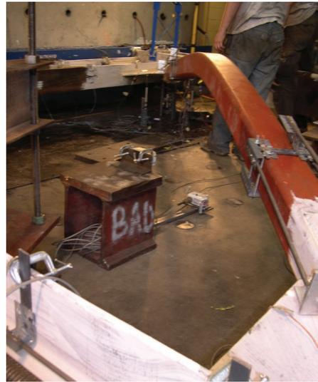
(b) Large out-of-plane deformation
