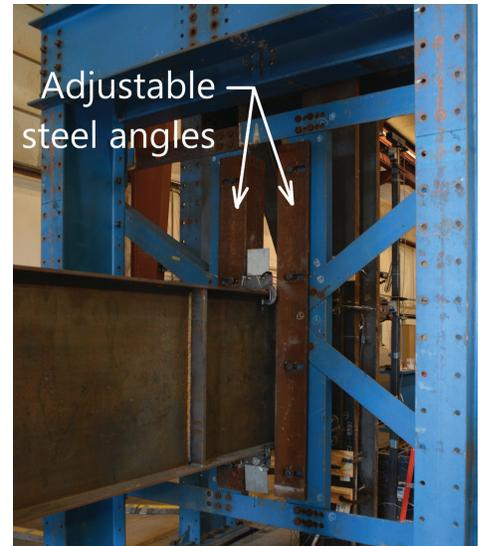
Fig. 4. Beam lateral bracing.
