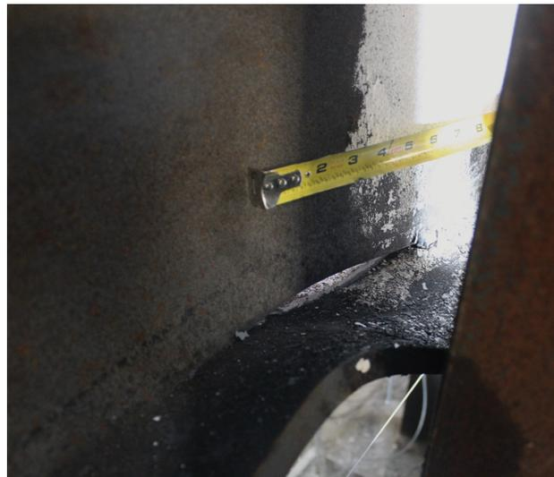
criteria similarly showed buckling over larger lengths (Blumenbaum and Murray, 2004). The larger zone of local buckling either caused or was exacerbated by the fracture of the weld joining the beam web and flange for Specimen 4E-1.5-1.75-36b.
