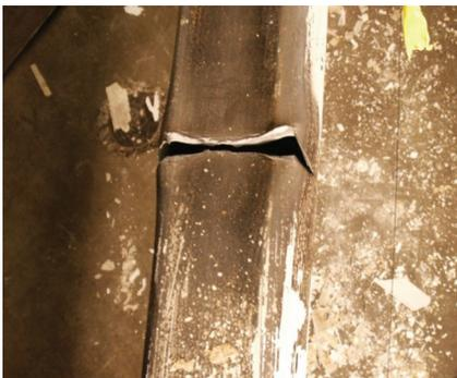
(e) Ductile tearing initiates at corners and progresses across the tube wall
